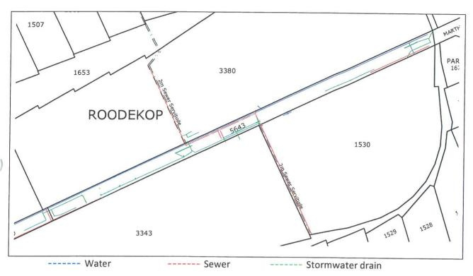
The water line runs parallel to the northern boundary of the site. A servitude can be registered to protect this line
